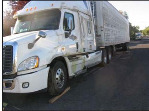
The 2009 Freightliner Cascadia truck was equipped with **RollTek**®, which kept the driver securely in his seat and inflated an airbag to cushion his head and neck from impact when the truck rolled over.
